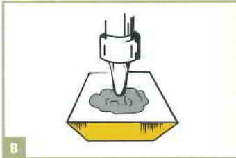
B Apply epoxy to the bottom of the marker, spreading evenly.
