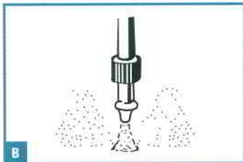
B Prepare the surface by removing any loose materials from the road surface.
