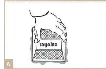
A Road surface should be dry. Place marker on the prepared road surface applying slight pressure until the marker contacts the road surface and forces a bead of epoxy or bituminous around all four corners.
